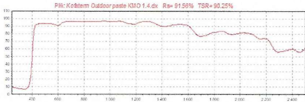
Fig. 1. The spectrum in the solar radiation range of the coating Kofaterm Outdoor Paste
